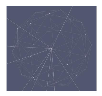
At right is an element with ordinary VTK node winding. Notice that (from the outside) the numbering can go clockwise or counter-clockwise, and that its outside direction reverses for the opposite face.
