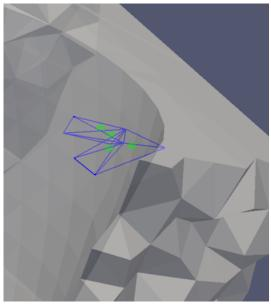
The picture at right shows the Lifted panel upon opening the mesh file. The tetrahedral analysis involves fewer edit boxes than the hex equivalent, and the unused ones are grayed out. The Verdict Edge Ratio attribute is the only one we seek, and the acceptable maximum level is 3.0 according to the standard.
